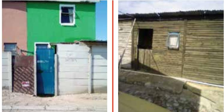
Figure 8: Typical freestanding backyard structures and main house extensions made of timber panels.
